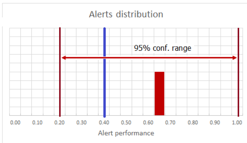
Fig. 2 - The blue line represents the performance of a naïve alert; the brown alert [1; 0] has a better performance, but it is NOT confirmed due to data insufficiency (its confidence range is too wide and includes the performance of a naïve alert)
