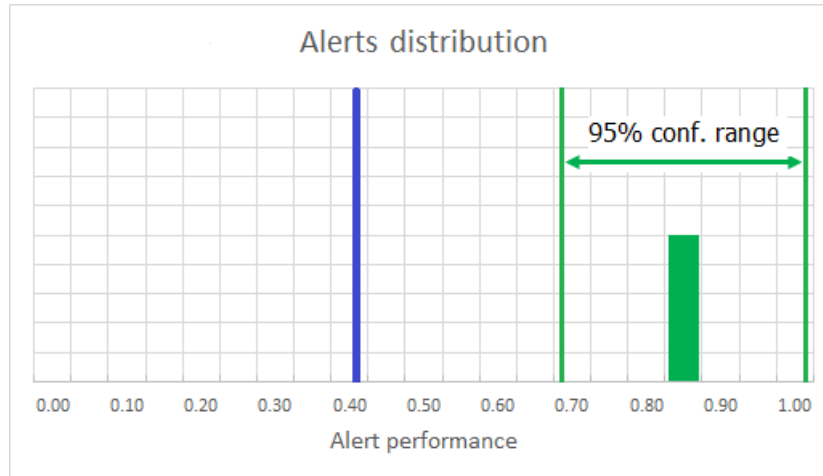
Fig. 1 - The blue line represents the performance of a naïve alert; the green alert [12; 1] has a better performance and its confidence does not include the performance of a naïve alert
